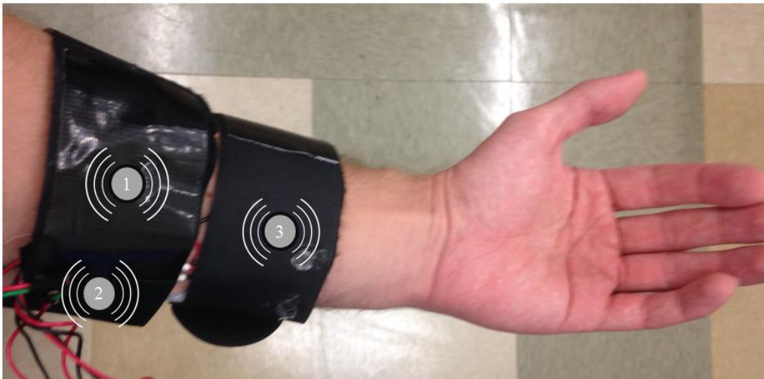
Figure 2.5: Motor arrangement for haptic setup 4. Motors are actuated based on numeric labeling smallest to largest.
